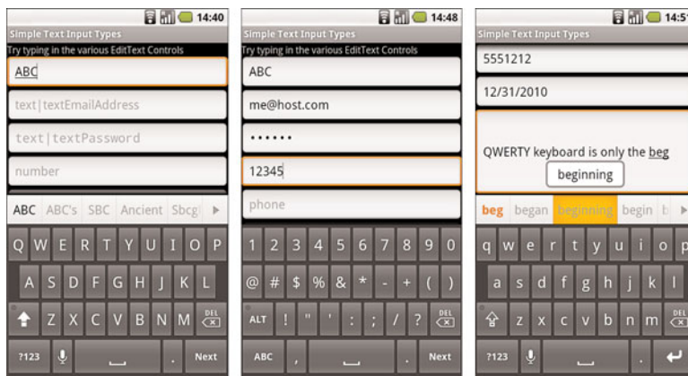
Figure 24.2 The software keyboards associated with specific input types.
