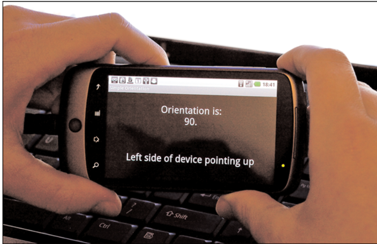
Figure 24.7 Orientation of the device as reported by an OrientationEventListener .
