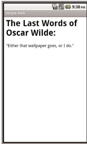
Figure 13.1 A WebView control used to display HTML.
