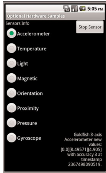
Figure 19.1 Sensor sample application showing accelerometer values.
