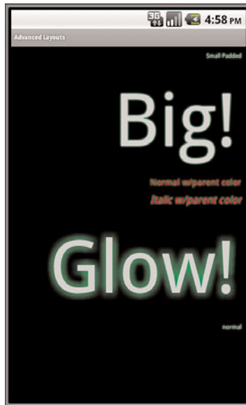
Figure 7.12 Packaging styles for glowing text, padding, and alignment into a theme.
