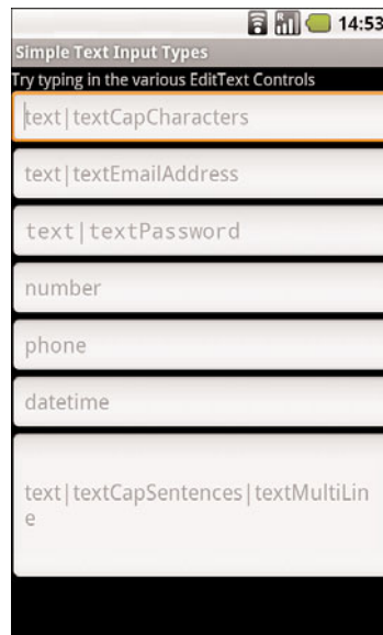
Figure 24.1 EditText Controls with different input types.
