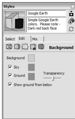
Figure 9-7: Use the Background section to turn on the sky and the ground, and to choose colors.
