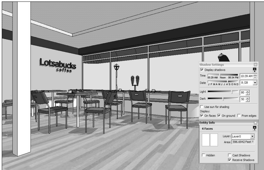
Figure 9-16: Tell the ceiling not to cast a shadow.
