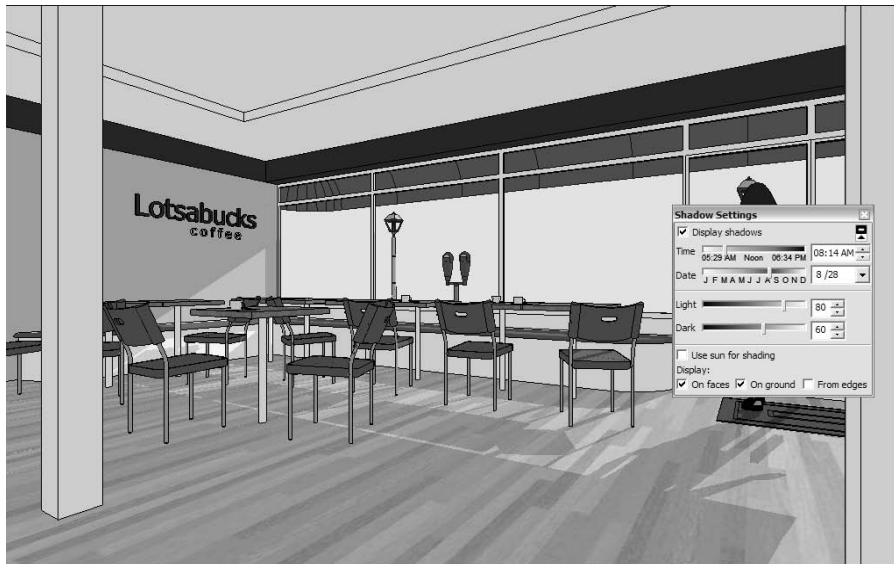
Figure 9-15: Brighten the room by decreasing the Dark setting.
