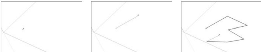
Figure 2-12: Use the Line tool to draw edges.
