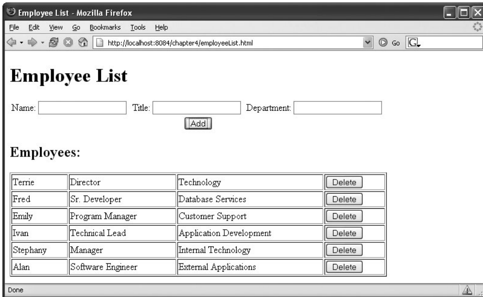
Figure 4-14. Each name is dynamically added to the list each time the Add button is clicked, without refreshing the page each time.
