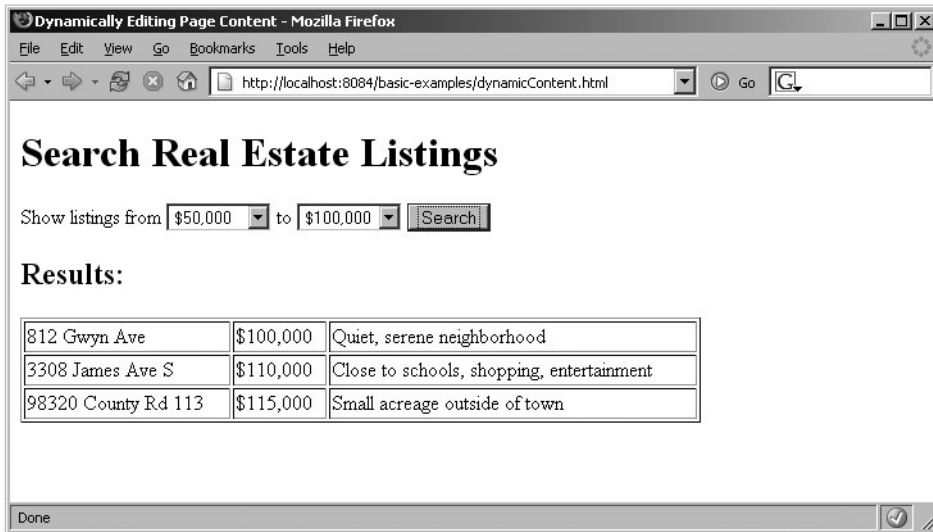
Figure 3-3. The results of the search were created dynamically using W3C DOM methods and JavaScript.
