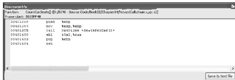
Figure 4-4: Small C++ code changes can result in large assembly- code changes.
