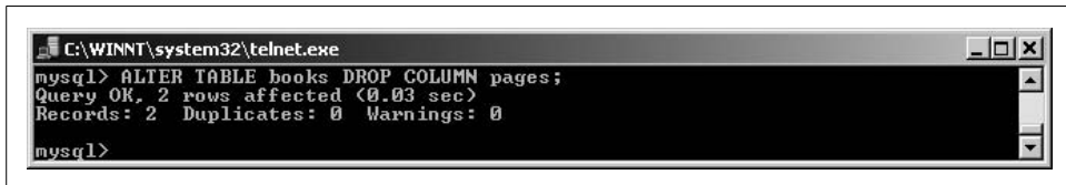
Figure 7-14. Removing a column
