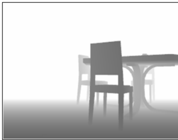
FIGURE 12-9 The Kinect depth sensor view from the robot.
