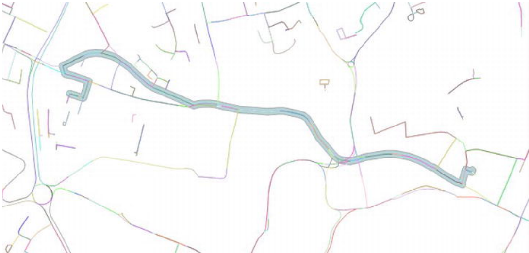
Figure 14-9. The A* route calculated between two nodes in the Norwich road network
