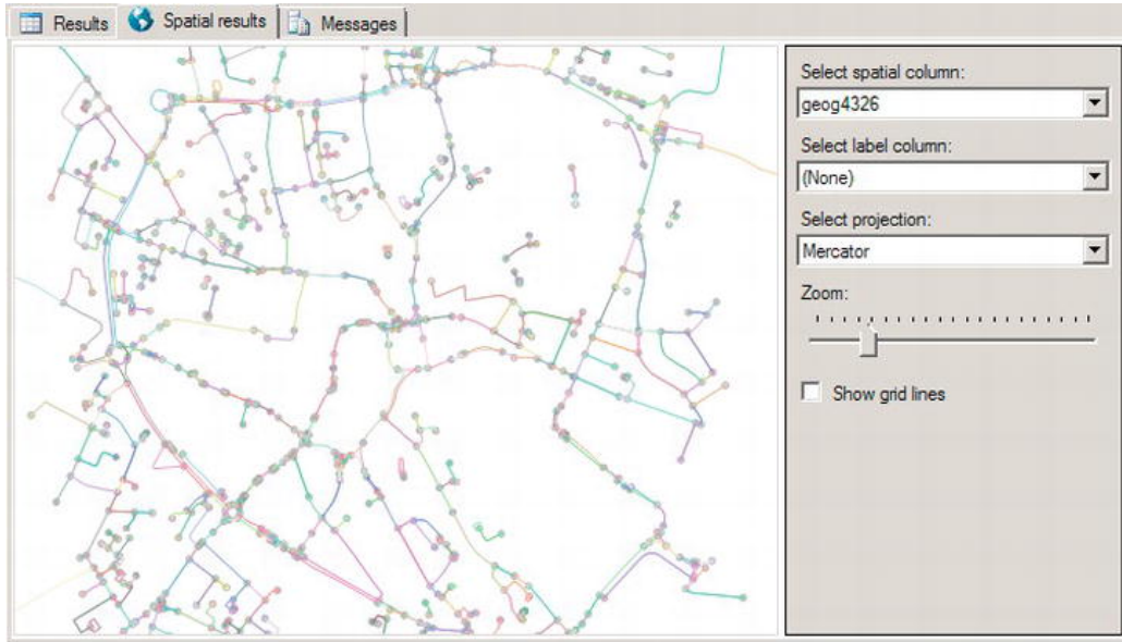
Figure 14-8. Nodes and Edges forming the Norwich road network
