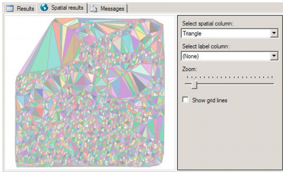
Figure 15-8. The 3D surface created by the GeometryTriangulate3d method
