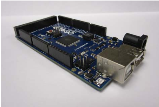
FIGURE 10-2: A close up view of the Arduino ADK board
