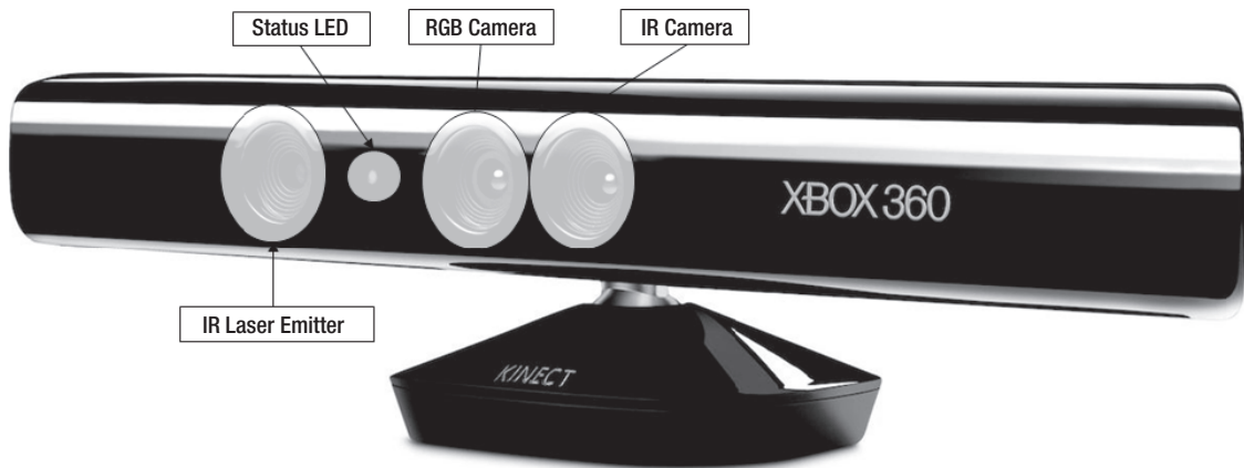
Figure 2-1. Kinect external diagram
