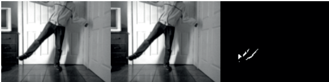
Figure 4-12. Image 1, image 2, and image 3 showing the frame difference using the depth camera
