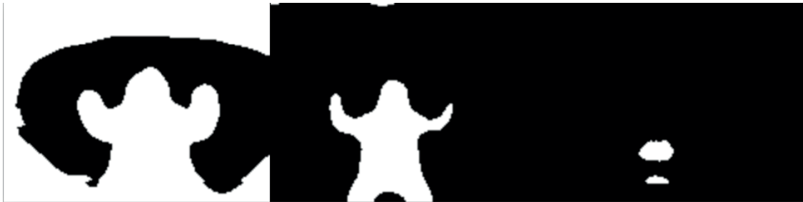
Figure 4-6. Tolerance too low (left), tolerance too high (center), and tolerance at the correct level (right)
