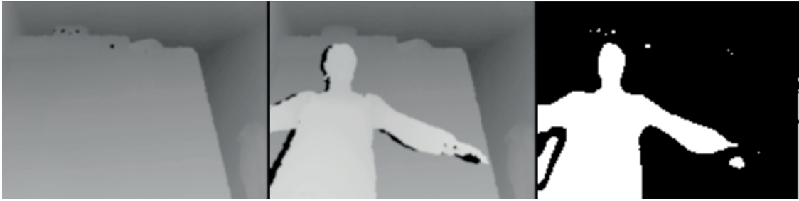
Figure 4-9. A background depth image (left), the same depth image with a person in it and lighting changes (center), and the resulting image (right)
