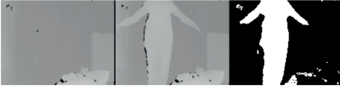
Figure 4-14. Background subtraction combined with frame differencing image
