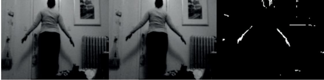
Figure 4-11. Frame differencing failing when the user is wearing a white shirt in front of a white background
