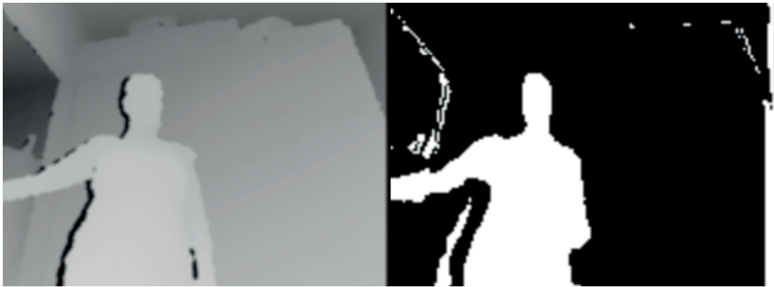
Figure 4-2. A greyscale image from the camera (left) and a black-and-white image that has been simplified by image processing to highlight the focus(right)
