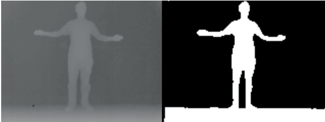
Figure 4-5. Kinect brightness image
