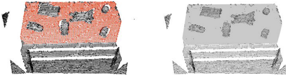
Figure 9-3. Left: Inliers detected as part of the table plane. Right: Estimated plane cropped to the table border using the convex hull of the inliers.
