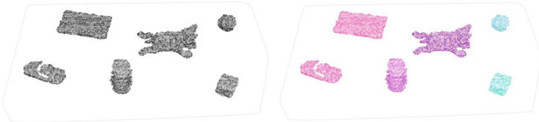
Figure 9-4. Left: Object points detected as lying over the table. Right: After clustering, each object has its own point cloud, materialized by a different color.
