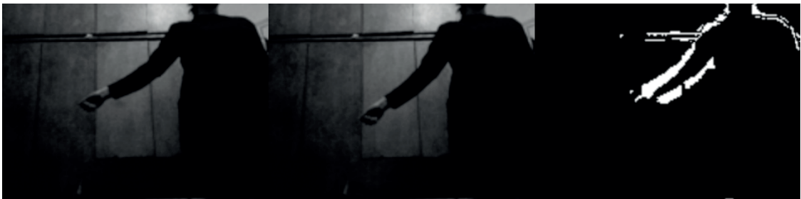
Figure 4-10. User with a hand raised (left), with a lowered hand (center), and the difference (right)
