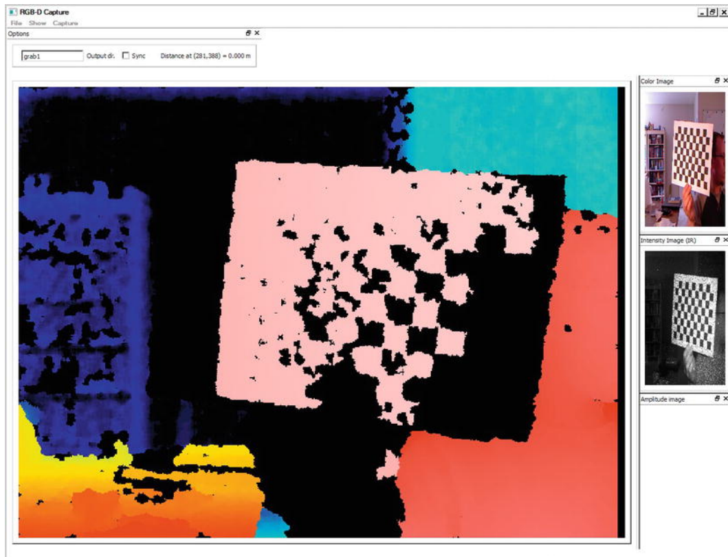
Figure 2-5. An example of a calibration position
