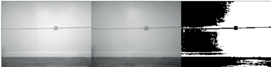
Figure 4-8. A background image (left), the same scene with lighting changes (center), the resulting image (right)
