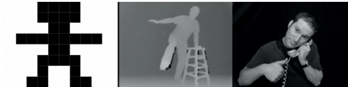
Figure 4-1. Icons (left) can be as small as 8 \times 8 pixels (64 total pixels). A 1024 \times 728 resolution image (right) has 745,472 pixels. The Kinect RGB and depth cameras (center) are both 640 \times 480 (307,200 pixels).
