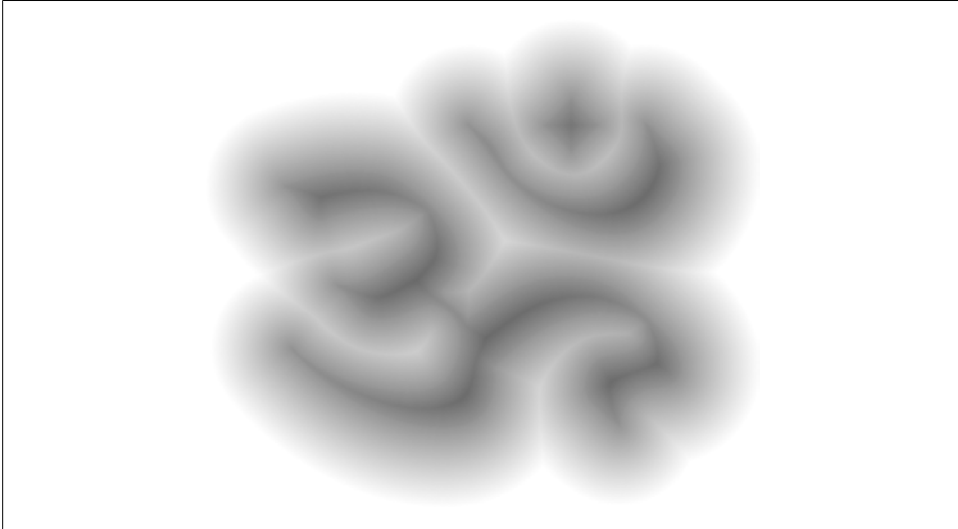
Figure 7-6. Signed distance field for the Aum symbol
