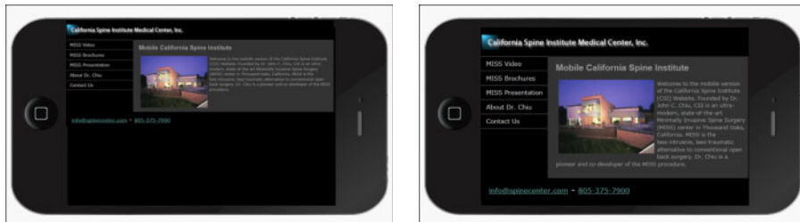
Figure 12-1: Example of page forced to fit the screen with viewport.
