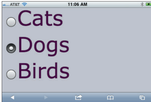
Figure 14-5: Radio buttons store whether a button is checked or unchecked.
