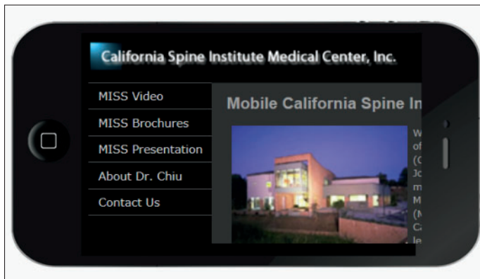
Figure 12-2: Example of mismatched screen redraw after changing phone ori- entation.
