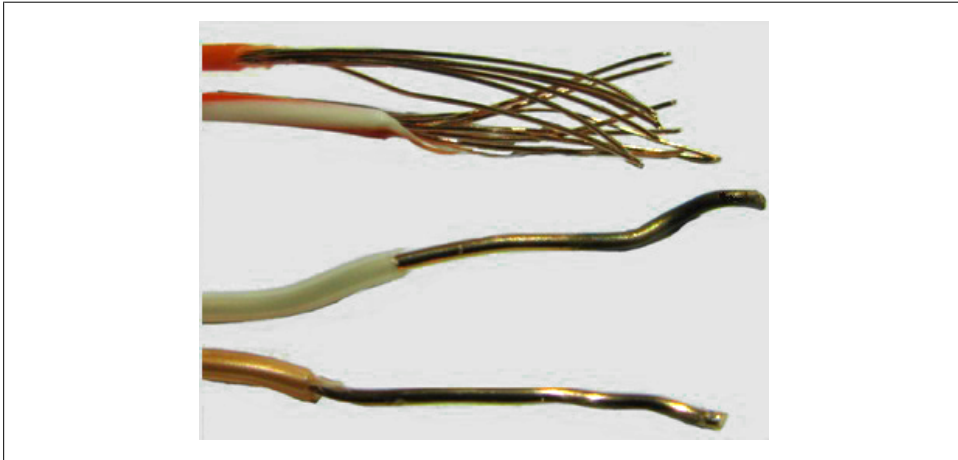
Figure 2-17. Stranded vs. solid core cable
