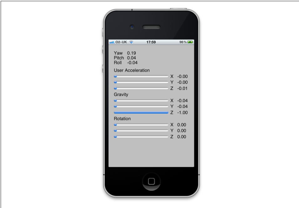
Figure 6-6. The Motion application running on an iPhone 4 sitting flat on the desk, with gravity in the negative Z-direction without any rotation or user acceleration
