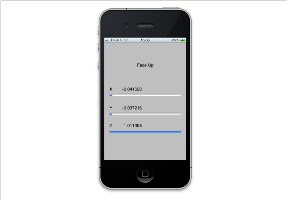
Figure 4-6. The Accelerometer application reporting the device orientation
