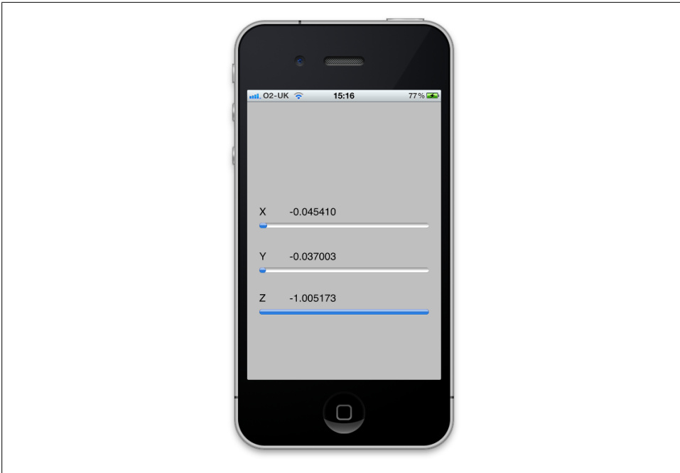
Figure 4-4. The Accelerometer application running on an iPhone 4 sitting face-up on my desk, measuring a 1-gravity acceleration straight down
