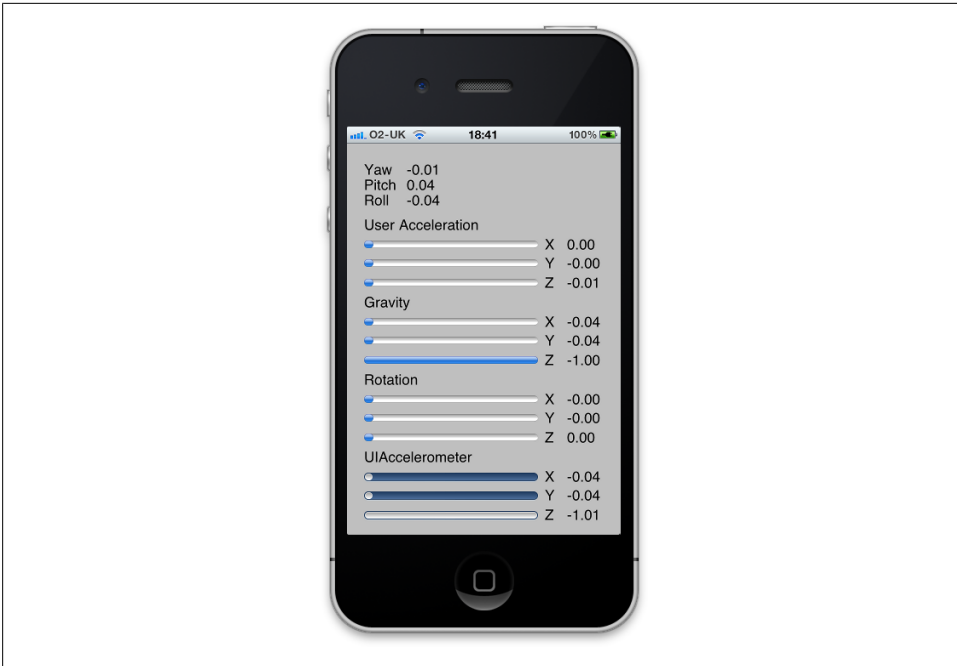
Figure 6-8. The Motion application running on an iPhone 4 sitting flat on the desk
