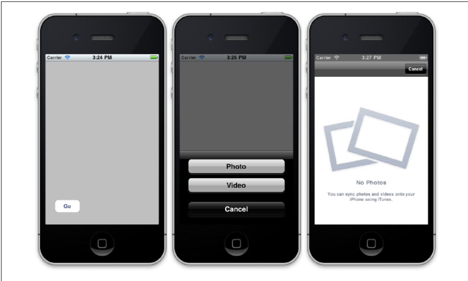
Figure 2-3. The initial Media application interface (left), the UIAlertController that pops up when the button is pressed (middle), and the Saved Photos folder that appears when the camera is unavailable (right)
