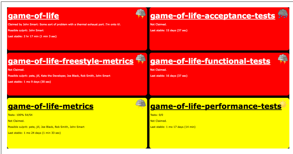
Figure 8-8. Displaying a build radiator view
