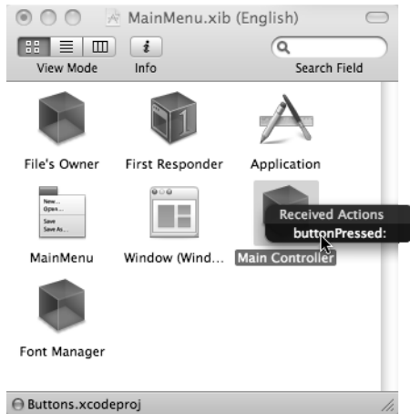
Figure 3–17. Connecting actions is very similar to connecting outlets. Ctrl-dragging to the controller class brings up a popup menu with all available actions.
