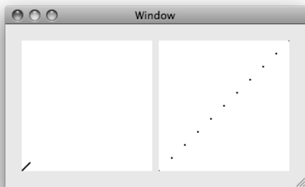
Figure 13-2. On the left, plotting points from a narrow range in a view with default bounds. On the right, the same points plotted in a view with smaller bounds.
