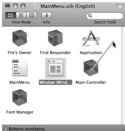
Figure 3-14. Ctrl-dragging from an icon in the nib's main window to an object on the user interface is how we connect an outlet to an object on the user interface.
