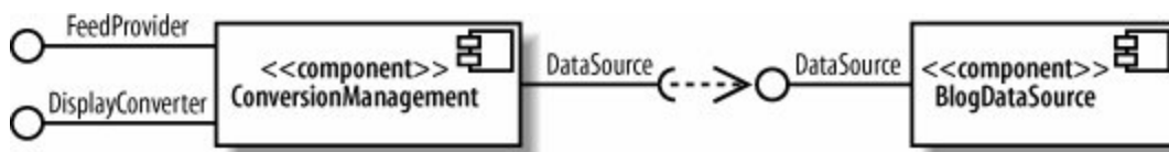
Figure 12-7. The ConversionManagement component requires the DataSource interface, and the BlogDataSource component provides that interface
