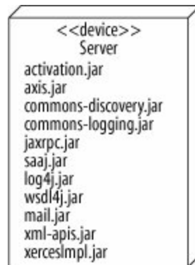
Figure 15-9. Listing artifact names inside a node saves a lot of space compared to drawing an artifact symbol for each artifact
