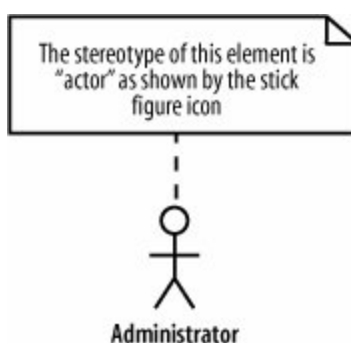
Figure 1-10. The Administrator is represented in the role of an actor because it is using the stick figure notation associated with that stereotype
