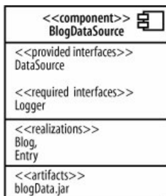
Figure 12-14. You can also list the realizing classes inside the component
