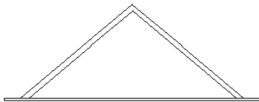
Figure 4-10: Part of a portico over a window, drawn using relative Cartesian and polar coordinates in architectural notation.
