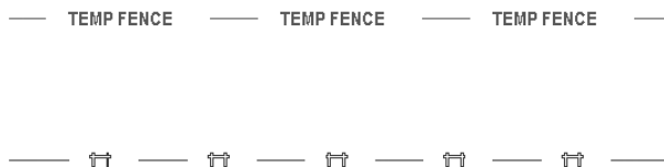
Figure 31-3: Complex linetypes include shapes or text.
