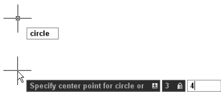
Figure 3-5: The Dynamic Input tooltip prompts you for input and then displays your input as you type.
