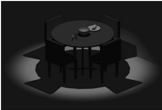
Figure 25-3: A rendering with one spotlight overhead. Here the hotspot angle is 45° and the falloff angle is 70°.
