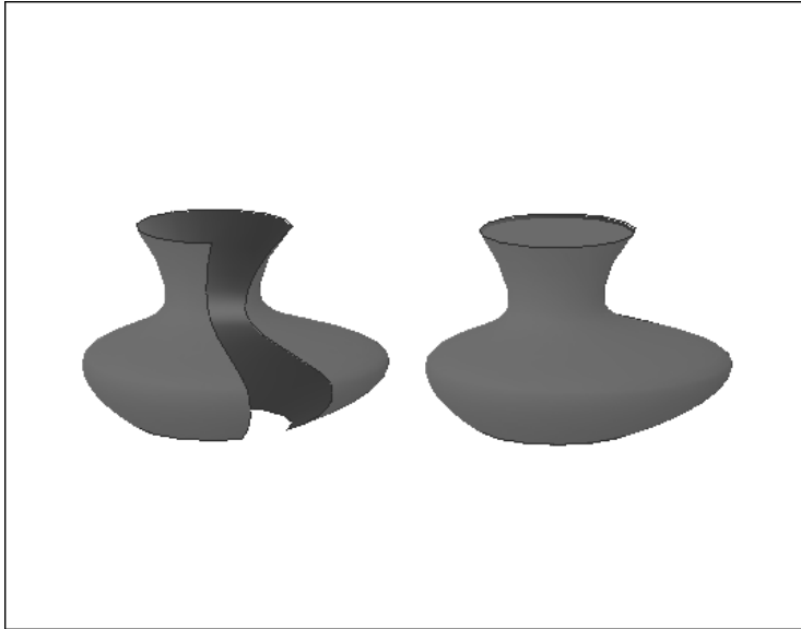
Figure 23-37: You can create either a surface or a solid with the LOFT command.
