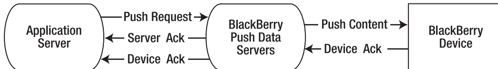
Figure 12–4. BlackBerry Push Service Plus delivery and acknowledgements
