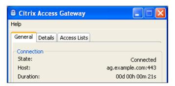
Should the user not belong to the correct group, then authorization will fail. We can view the effects from the **Connection Status** tab of the CAG plug-in; the **Access Lists** tab will be missing.
