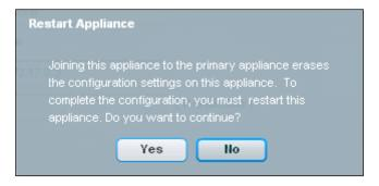
Both gateways, master and slave, need to reboot. We should ensure that the master device reboots first, so as not to cause a failover. We can confirm the running settings on the **Monitor** tab; now we will have the happy green tick indication that we have set up appliance failover. The setting up of appliance failover is shown in the following screenshot:
