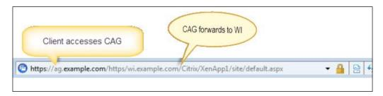
In short, using the CAG will allow for secure remote access to internal resources without the use of additional IP addresses or opening up ports other than HTTPS/443 through the Internet-facing firewalls.
