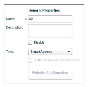
From this, we can also see that, when using **SmartAccess** logon points, authentication must occur at CAG and cannot be passed through to the WI server.
