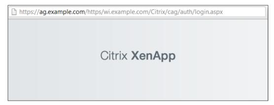
At this stage, we will not be able to authenticate, but we have proved the validity of the configuration so far. You may also like to access the WI website without using the CAG. The Citrix WI server is located on our private network and there is no route to it using either its DNS name or IP address. Access can only be achieved by using the CAG.
