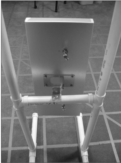
Figure 8-4: A home-made, freestanding PVC antenna rack.
