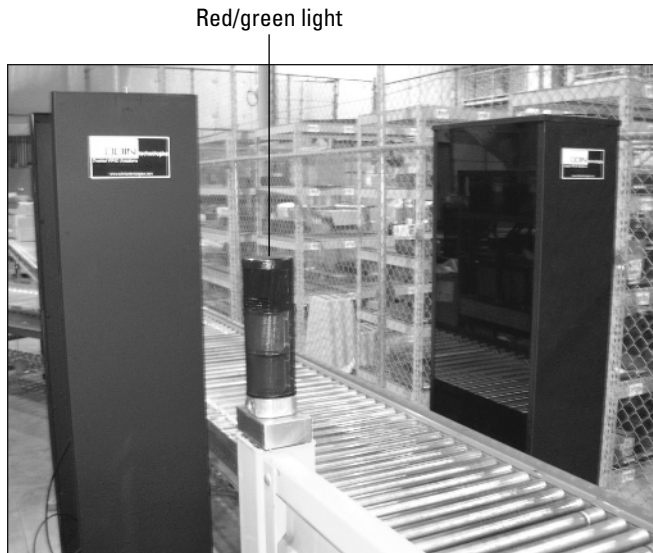
Figure 13-2: A light stack that provides a green light signal if an item is successfully scanned.
