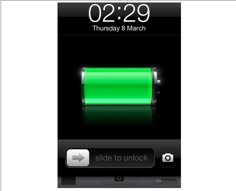
Figure 1-14. An example of a trigger. In iOS (as in Windows Mobile), you can use the camera even on a locked phone. Pressing the camera icon bounces the bottom bar up a little, indicating that you swipe up to get the camera functionality. Of course, slide to unlock is its own trigger as well.
