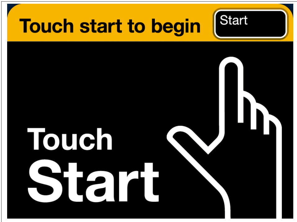
Figure 2-1. The idle screen from the MetroCard Vending Machine. Antenna Design deliberately overemphasized the trigger, which was not, as one might suspect, the button in the top right. It’s actually the whole screen. (Courtesy Antenna Design.)
