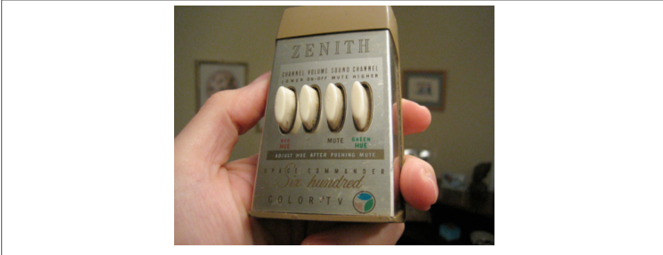
Figure 1-11. Although there had been remote-control planes and boats previously (mostly for military use), the Space Commander television remote removed proximity from control for consumers. (Courtesy Peter Ha.)
