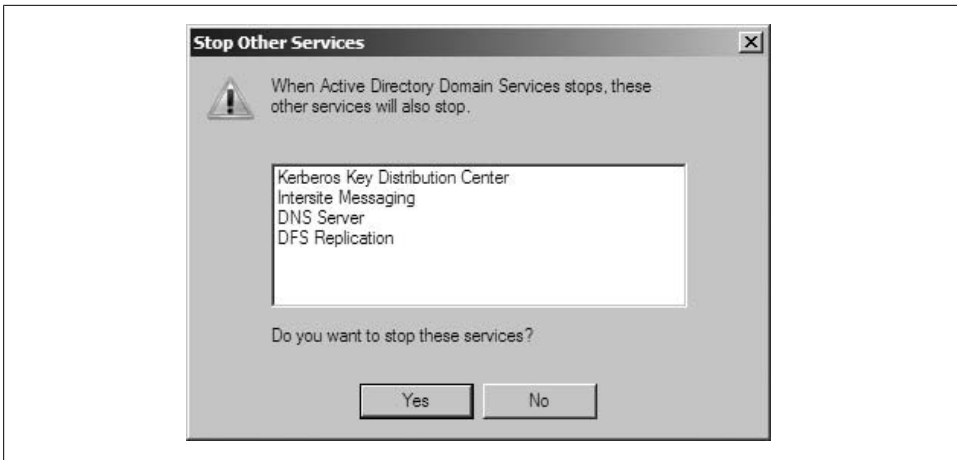
Figure 15-17. Stopping the Active Directory service
