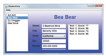
The ListBox on the left lists the students in the Students table. When you click on a student, the controls in the middle display the student's address and phone number, and the ListBox on the right displays the corresponding test score data from the TestScores table.
