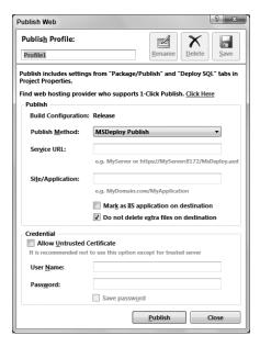
Because many developers are continually deploying their Web applications to their testing, staging, and production environments, there is a capability to store your deployment options in a profile that you can use again and again. Also notice in the dialog in the previous figure that the build configuration is set to Release for this deployment. This setting comes from what you have set in the toolbar of Visual Studio 2010 before you select the Publish option.
