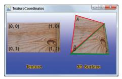
The picture on the left shows the texture material with its corners labeled in the U-V coordinate system.
