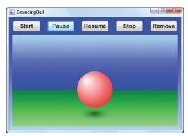
The second Parallel Timeline contains two Double Animation Using Keyframes objects, one to control the ball's Canvas. Top property and one to control the shadow's Opacity. As the ball's animation moves the ball downward, the shadow's animation makes the shadow more opaque. When the animations end, the ball is touching the "ground," and the shadow is fully opaque.
