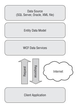
As you can see from this figure, the WCF Data Services layer is not the layer that interacts with the database. Instead, you are working with an EDM layer that is the mapping layer between the data store and the cloud-based interface. When working with your EDM, you are able to use LINQ to SQL and LINQ to Entities.
