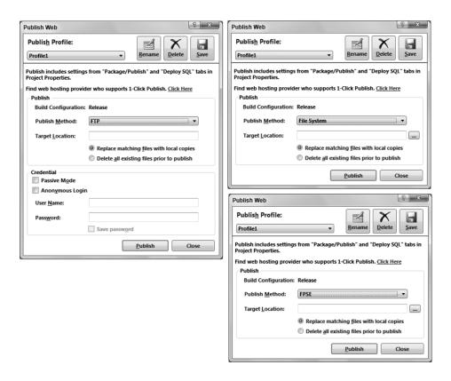
In this figure you can see some standard settings for doing deployments using FTP, the file system, or FrontPage Server Extensions.
