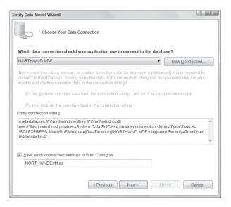
In the previous screenshot, notice that the connection string and the locations of the mapping details are going to be stored within the web. config file. You can also see on this screen that you are naming the instance of the model NORTHWNDEntities in the text box at the bottom of the wizard. This name is important to note because you will use it later in this example.
