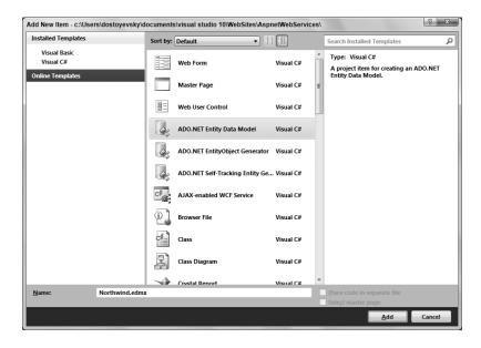
As shown in the figure, name your ADO.NET Entity Data Model file Northwind.edmx. When you create the Northwind. edmx file by clicking Add, the Entity Data Model Wizard appears, offering you the option of creating an empty EDM or creating one from a pre-existing database. For this example, choose the option to create one from the pre-existing (Northwind) database. Then click Next in the wizard.
