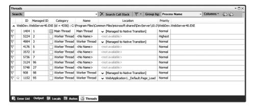
You can double-click on a thread and go to where that thread is in the code when debugging. You can also get a visual family tree view of the threads at work by opening up the Parallel Stacks dialog. The next figure shows this dialog.
