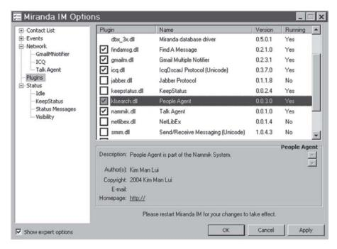
FIGURE 4.20 Plug-ins of Miranda IM are DLL files.
