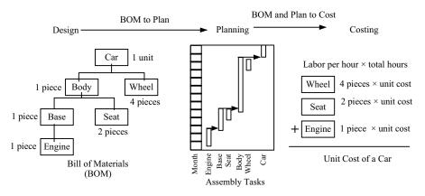
**FIGURE 1.1** How bill of materials (BOM) can be used for planning and costing.
