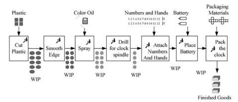
**FIGURE 8.15** An assembly line for producing clocks.
