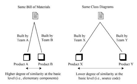
**FIGURE 1.3** *Degree of difference* is a conceptual term measuring how two products can be built differently using the same design.
