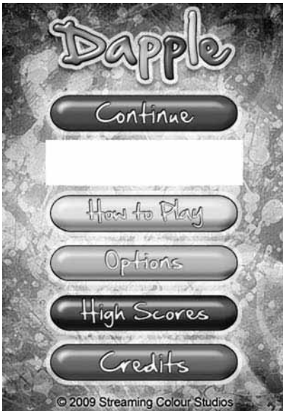
Figure 4-8. An example from Dapple of the strange behavior that can occur as a result of a memory stomp
