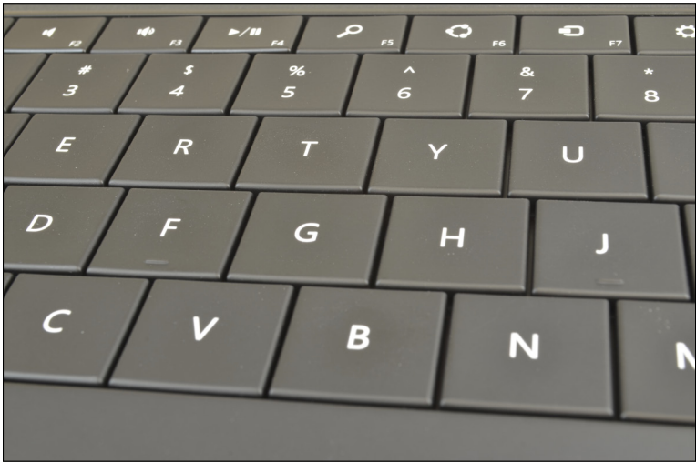
Figure 5-2: The Surface Type keyboard offers mechanical keys that move when touched.
