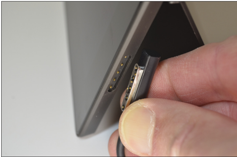
Figure 2-4: The symmetrical connector fits into the charger socket either way.
