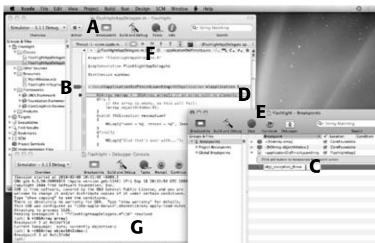
Figure 2-1: The Xcode debugger in action. You can enable or disable breakpoints using the toolbar icon (A). To set a breakpoint in your source code, click in the left gutter until you see a blue arrow (B). The Breakpoints window shows all the breakpoints that have been defined, and you can add new ones to the end of the list (C). When a breakpoint is reached, the line of source code will be highlighted (D), and you can easily navigate the stack back-trace with a pop-up menu (E). Controls are also available to step through code (F). More advanced operations can be performed in the debugger console (G).
