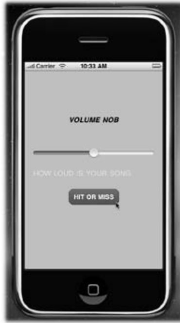
Figure 3-7: After connecting the outlets to the slider and label controls, the HitMakerViewController code in -viewDidLoad can update the position of the slider along with the label's text and color. When you launch the application now, nothing happens if you try clicking the button or slider.
