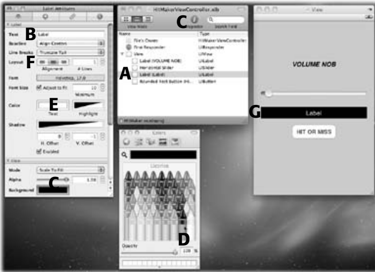
Figure 3-11: Adjusting the colors and layout of the second label. Select the label (A) and then go to the Attributes Inspector (B). Click the Background color well (C), and select a black background (D). You can change the text color using its own color well (E). You adjust text alignment using the Layout control (F). The results are shown in the View window (G).
