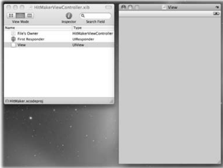
Figure 3-3: Here's the blank palette you're going to working with. The document window is on the left, and the application's only view is on the right. Note that the View listed in the document window doesn't have any children (subviews) yet.
