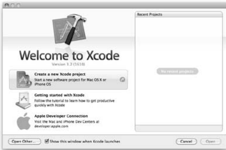
Figure 1-6: The Xcode launch window. As you create new projects with Xcode, you see them listed on the right. Click the “Create a new Xcode project” button to start your first iPhone application. The “Getting started with Xcode” button opens the documentation viewer and displays a helpful overview of Xcode. The last button is a convenient link to the Dev Centers for the Mac and iPhone.
