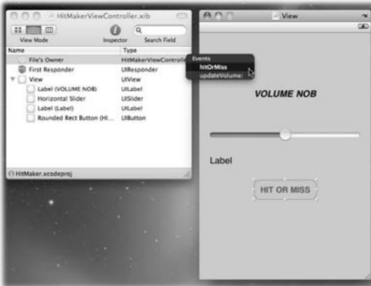
Figure 3-8: After dragging a connection from the HIT OR MISS button to the HitMakerViewController , you'll select the hitOrMiss action. This move causes the named method to be called when the button is pressed.
