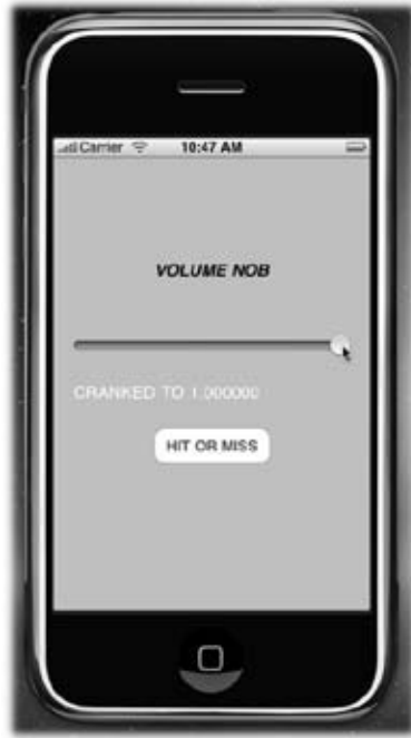
Figure 3-10: When you run the application, the slider and button controls now function, but some problems linger. The slider control value only goes up to 1.0, the contrast for the label is too low, and the text isn't aligned correctly. You can fix all of these bugs with Interface Builder.
