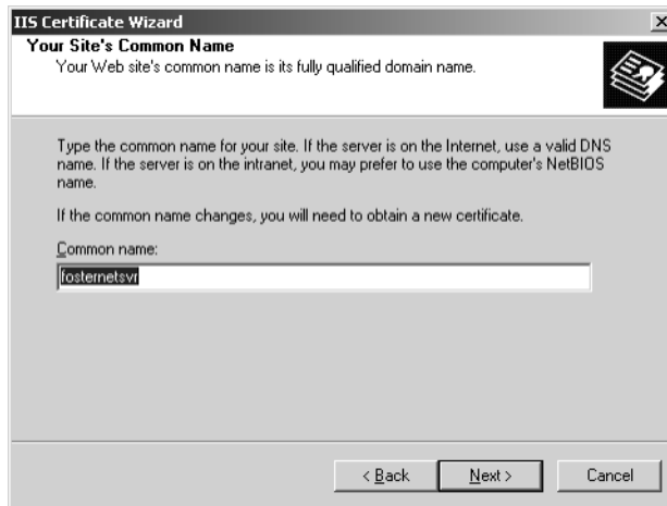
Figure 9.6 Assign a common site name.
