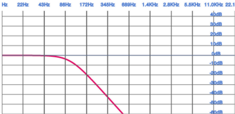
Figure 6-1. Frequency response graph for a low-pass filter
