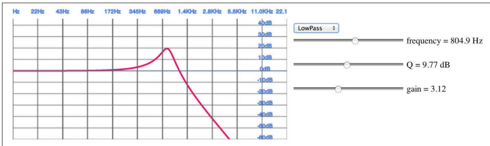
Figure 6-2. A graph of the frequency response of a low-pass filter with parameters
