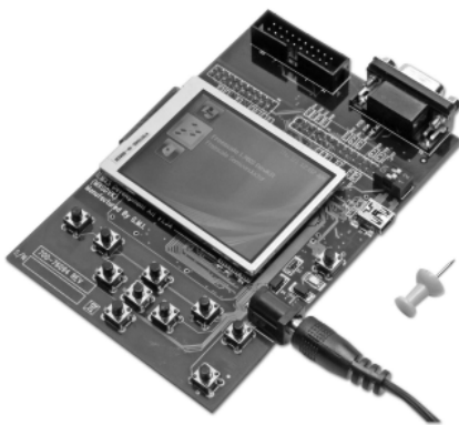
Figure 1-3. A .NET Micro Framework development board (copyright of Freescale Semiconductor, Inc. 2008, used by permission)
