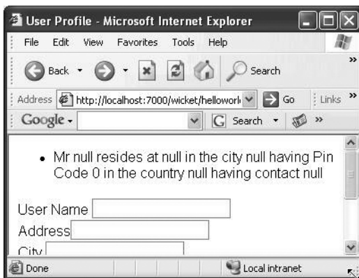
Figure 2-4. The UserProfilePage allows “blank” input values in the absence of a validation check.
