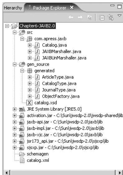
Figure 6-12. Schema-derived Java content classes generated by xjc
