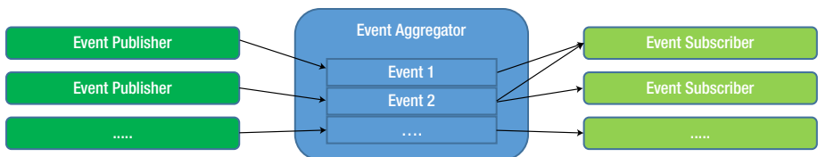
Figure 4-1. An Event Aggregator Service Supporting Pub/Sub Model for Events/Messages
