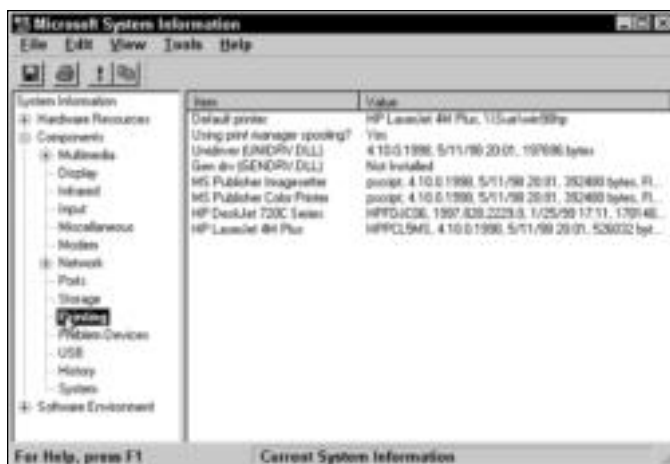
Figure A-4: View information about your system components.
