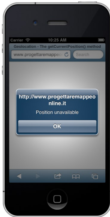
Figure 6-3. Example of an error message generated by analyzing the code property of the PositionError object. In this case, the error code was POSITION_UNAVAILABLE (numeric value 2)
