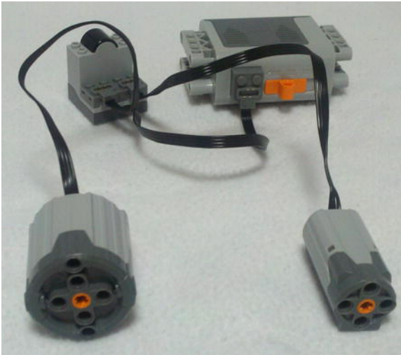
Figure 3-6. This is the type of setup you will need if you want both steering and motion on your Technic creation. Figuring out how to integrate them in your creation may be the hardest part of building.
