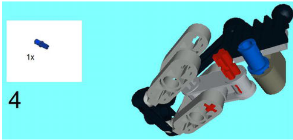
Figure 5-27. Place a Connector Peg/Cross Axle in the Cross and Hole 2M Beam. I realize that I usually don't spend one step on one particular part, but I found that the 2D views of this 3D model were confusing, and I thought it would help the builder to see another angle.
