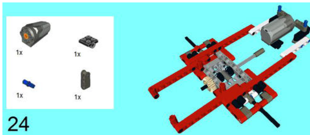
Figure 5-74. The steering engine (M-Motor) is plugged in to the front. Note how the 2x 2 Technic Bearing Plate is on the motor. With its hollow studs, it comes in about half a stud into the motor. This is similar to the rack and pinion steering column in Chapter 3.
