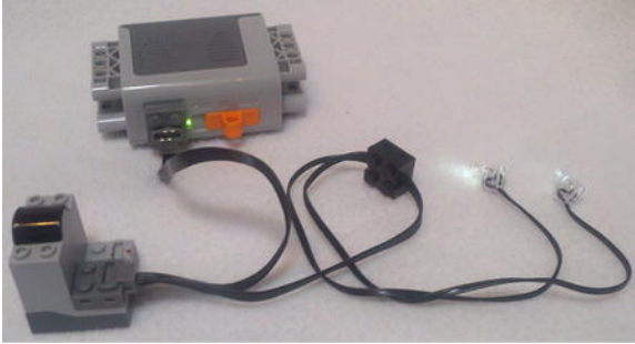
Figure 4-2. You could set up your lights this way with the IR-RX remote, but I don't recommend it.
