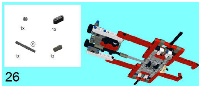
Figure 5-76. The central axle gets an extension and a 6M Axle. A Half Bush and 3M Beam get involved with the Technic Bearing Plates.
