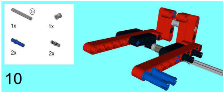
Figure 2-36. Except for the Connector Pins, the action of this step takes place with sliding the 5M Axle in between the two 4 x 2 Beams, with the Bush in the middle.
