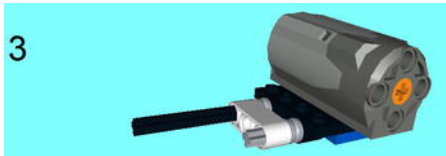
Figure 3-11. Instead of leaving a studded section, it is actually half of one. At this point, the pieces assembled in step 1 and step 2 now join up as shown, with 1M of both axes joining with the Technic Bearing Plate of the left side of the M-Motor.
