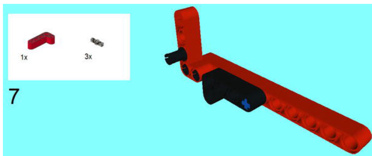
Figure 2-33. It is necessary to join a 4 x 2 Beam to this 11M Beam.
