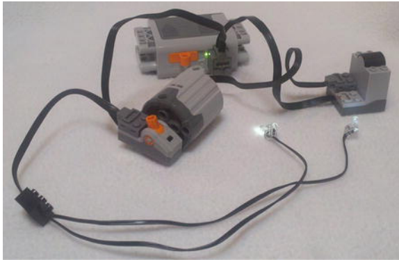
Figure 4-6. A very complex way of hooking up your lights so they will turn off by remote.
