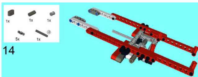
Figure 5-64. At this point, a 4M Axle joins the H-Frame with a Bush. A Cross Axle joins with the 12M Axle, and a Cross and Hole joins up here as well.
