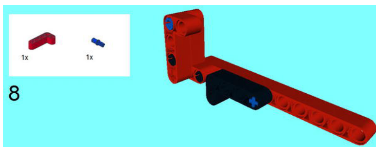
Figure 2-34. An inverted 4 x 2 Beam joins with this other one.
