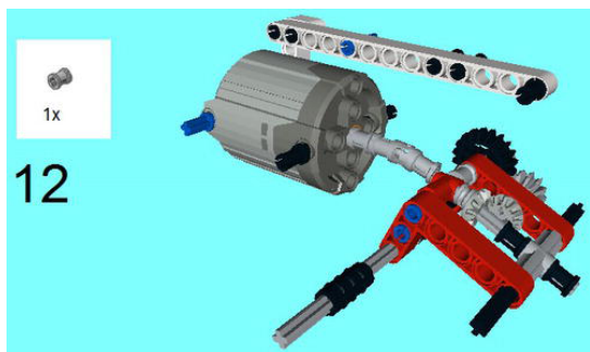
Figure 5-13. Join the separate creation of Steps 4-11 to the XL-Motor via a Bush.
