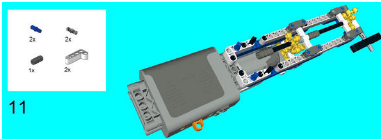
Figure 7-109. Add two 4 x 2 Beams to the structure. Even though you see an engine listed as one of the parts, all that is required here is to attach the other end of the connector. Also note the Cross Axle Extension.
