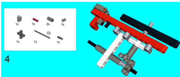
Figure 7-44. The 10M Axle joins with the Angular Gear and two Tubes with a Bush allow it to mesh together in a perpendicular method. The Cross Block joins with the 180 Degree Angle Element with a 2M Axle and Connector Peg.
