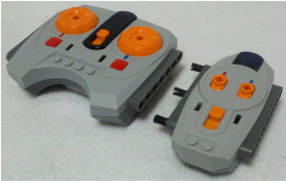
Figure 4-11. The mega remote, a way of using many features on your LEGO Technic creation. Simply push them together to get them to work.
