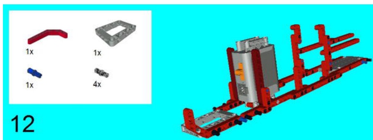
Figure 7-14. Add a 5 x 7 Beam Frame here with a Double Angular Beam.
