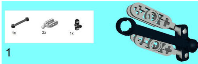
Figure 5-24. Two Steering Knuckle Arms connect to a Steering Arm via ball-and-socket connections. A 6M Track Rod attaches to the Steering Arm in the same ball-and-socket fashion.
