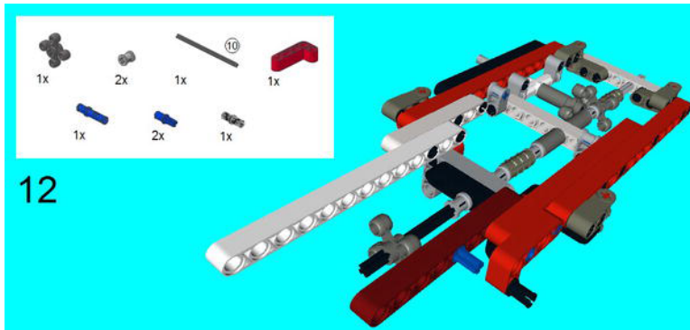
Figure 7-52. Add a 10M Axle along the center here, with a Bush and an Angular Gear. Add a 4 x 2 Angular Beam along the side.
