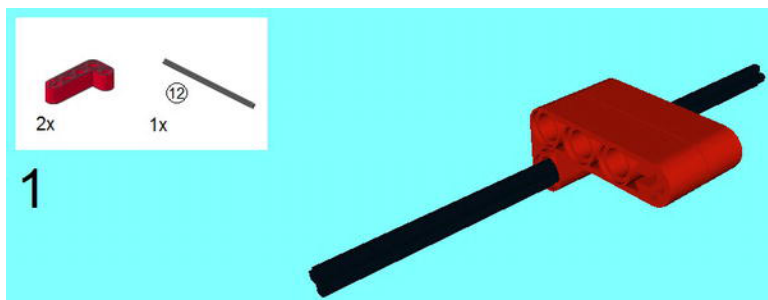
Figure 2-42. The first step in adding motorized wheels is to add two 4 x 2 Beams directly in the center of a 12M Axle.
