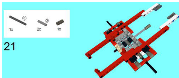
Figure 5-71. Two 3M Axles join here on the 180 Degree Element, along with a 6M Axle. Note the Cross Axle extension on the middle.
