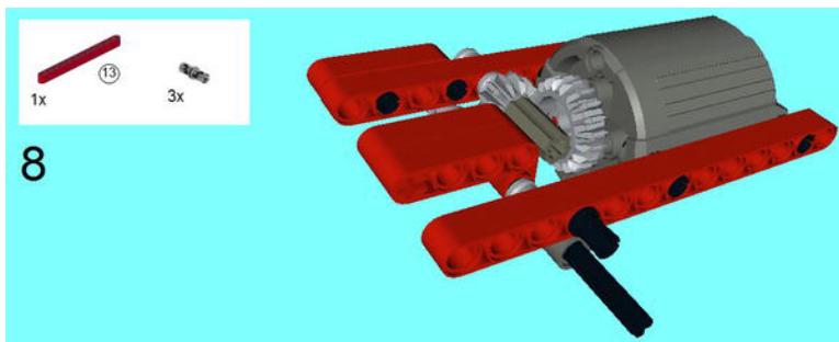
Figure 2-49. At this point, the construction can be turned around, and a 13M Beam gets put on with the Connector Pegs.
