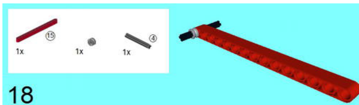
Figure 5-41. This is another separate creation. Start with a 15M Beam and add the 4M Axle with Half-Bush. Leave 1M of Axle exposed on the side with the Half-Bush.
