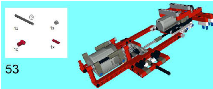
Figure 5-103. As you can see, the 6M Axle joins up with the XL-Motor and will help hold it in place.
