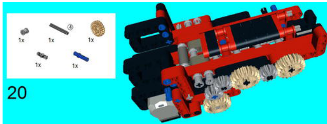
Figure 6-79. Add another Z20 Double Bevel Gear, 4M Axle, and Bush to mesh with the other Double Bevel Gears on this side. On the opposite side, add the Connector Peg and 3M Connector Peg.
