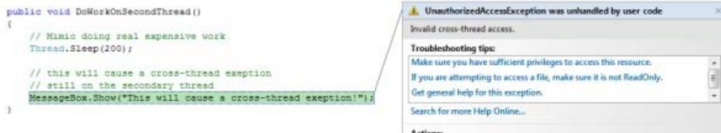
Figure 10-7. Invalid cross-thread access will occur when a secondary thread tries to manipulate UI objects created with the main application thread.
