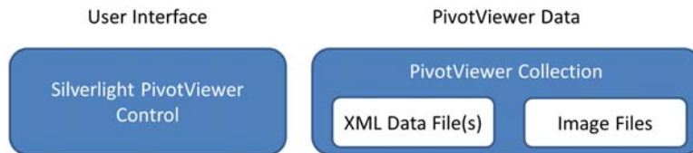
Figure 14-2. A PivotViewer module consists of the Silverlight PivotViewer control and the PivotViewer collection files.
