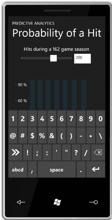
Figure 12-6. Setting input focus on the text block will cause a virtual keyboard to appear for user input. The control is formatted for number input, so it will default to numbers.
