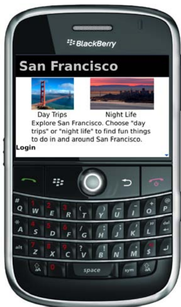
Figure 14–2. In this layout, note that to create even spaces around the images, the screen cannot use percentages for table widths.
