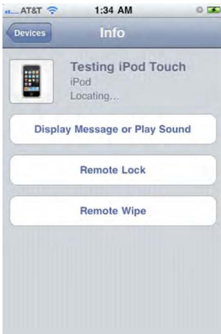
Figure 4–20. Remote locking and wiping iOS with Find My iPod
