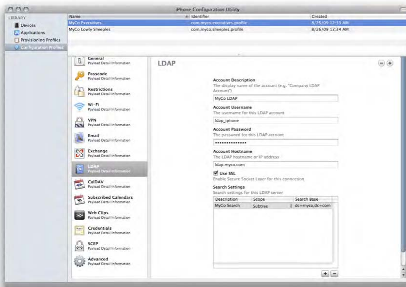
Figure 8–15. iPhone Configuration Utility: Configuring LDAP accounts
