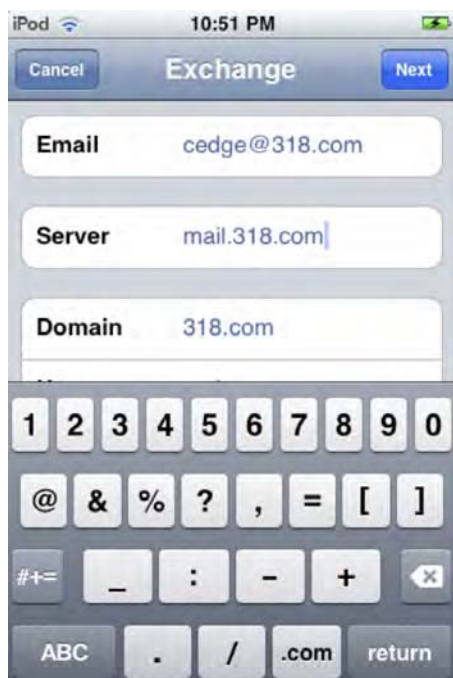
Figure 4–7. Adding a server when AutoDiscover fails
