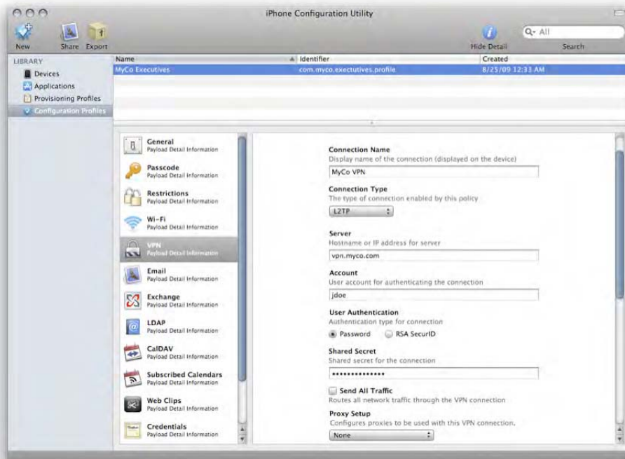
Figure 8–11. iPhone Configuration Utility: VPN configuration
