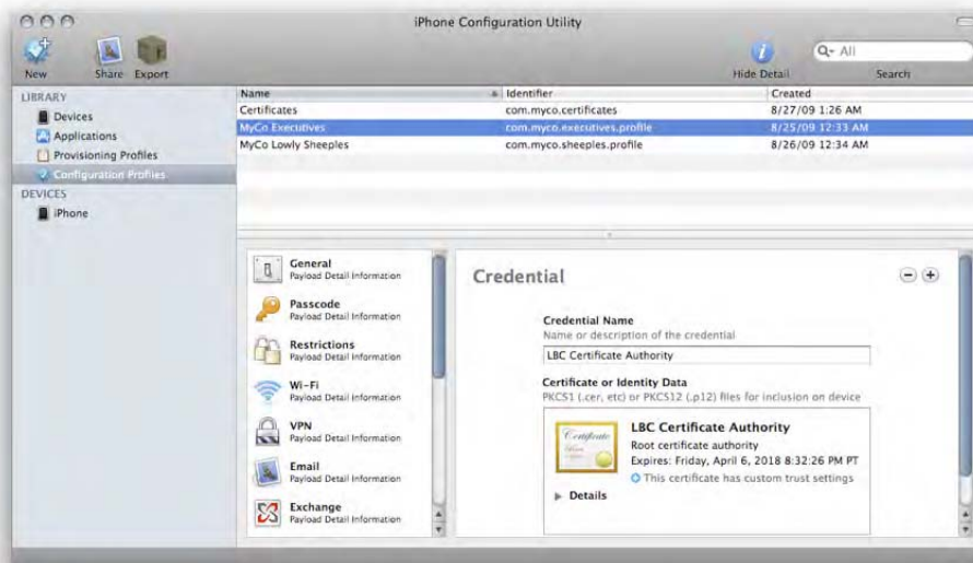
Figure 8–24. iPhone Profile Installation: Providing authentication credentials
