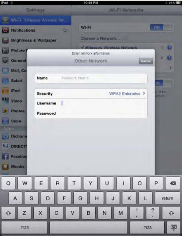
Figure 3–4. Configuring wireless access
