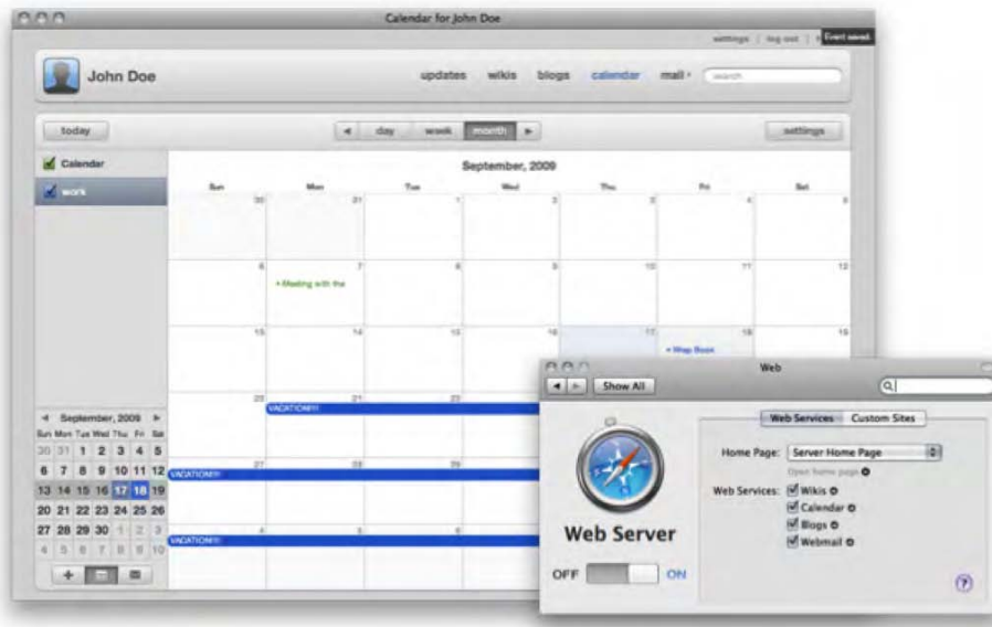
Figure B-9. Configuring Calendar Web Services in Server Preferences (front), Web Calendar Interface (back)
