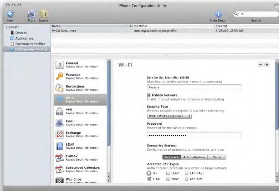
Figure 8–7. iPhone Configuration Utility: Wi-Fi
