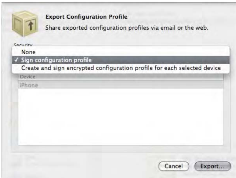
Figure 8–25. iPhone Configuration Utility: Signing a configuration profile
