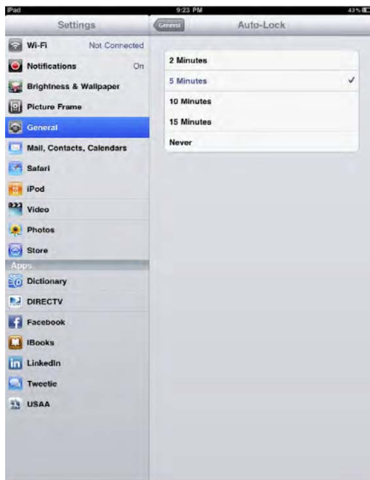
Figure 3–22. Setting time for passcodes
