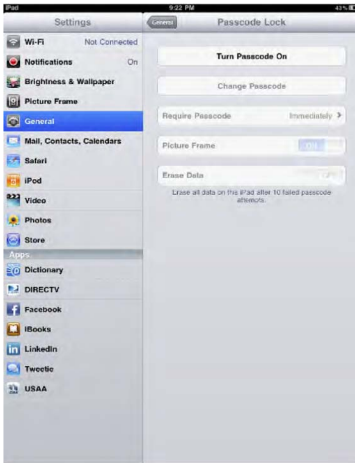
Figure 3–21. Enabling a passcode to access a device
