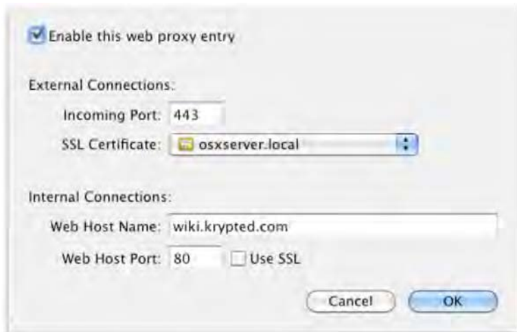
Figure 6–17. Enabling the Mobile Access web proxy
