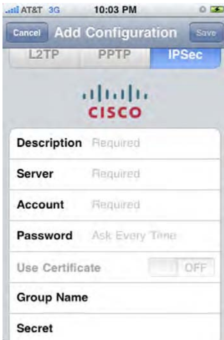
Figure 6–4. Standard Cisco VPN client settings
