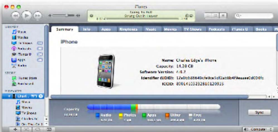
Figure 9–1. Obtaining the UDID of a device
