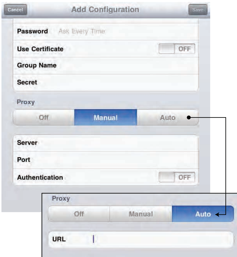
Figure 6–5. Proxy configuration for iOS
