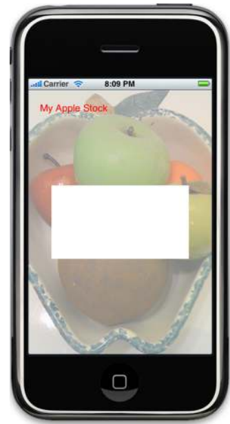
Figure 4.3 Combining graphics and text can be hard in some programming languages, but under the SDK it can be done entirely with Interface Builder. Here you see a background image with a text overlay.
