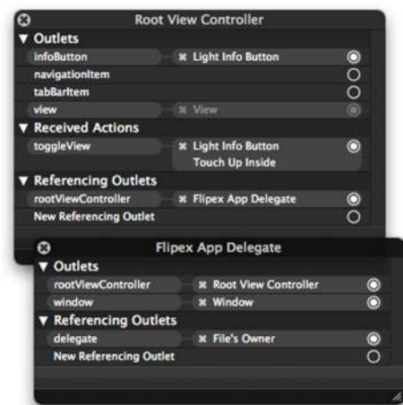
Figure 7.9 Objects in Interface Builder can connect to a variety of different files.
