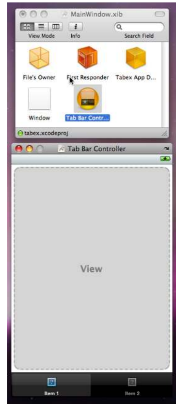
Figure 7.2 Dragging a tab bar controller to the nib display window creates the tab bar interface.
