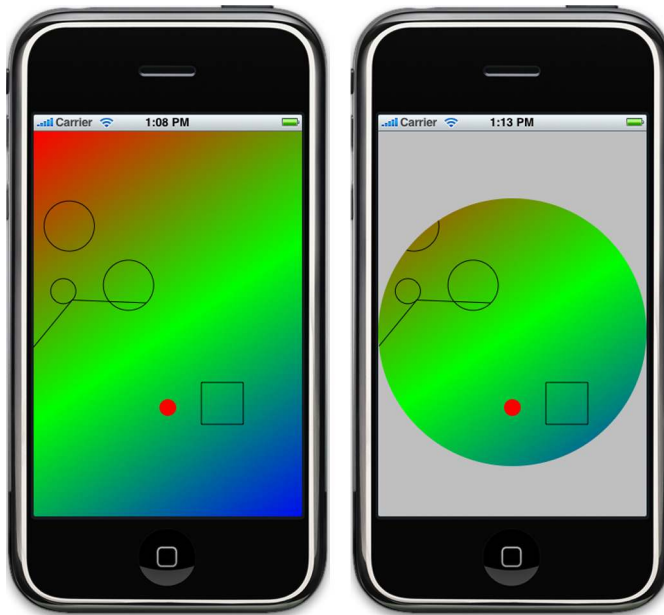
Figure 13.3 An example of a clipping path in use. The unclipped image is on the left, and the clipped image is on the right.
