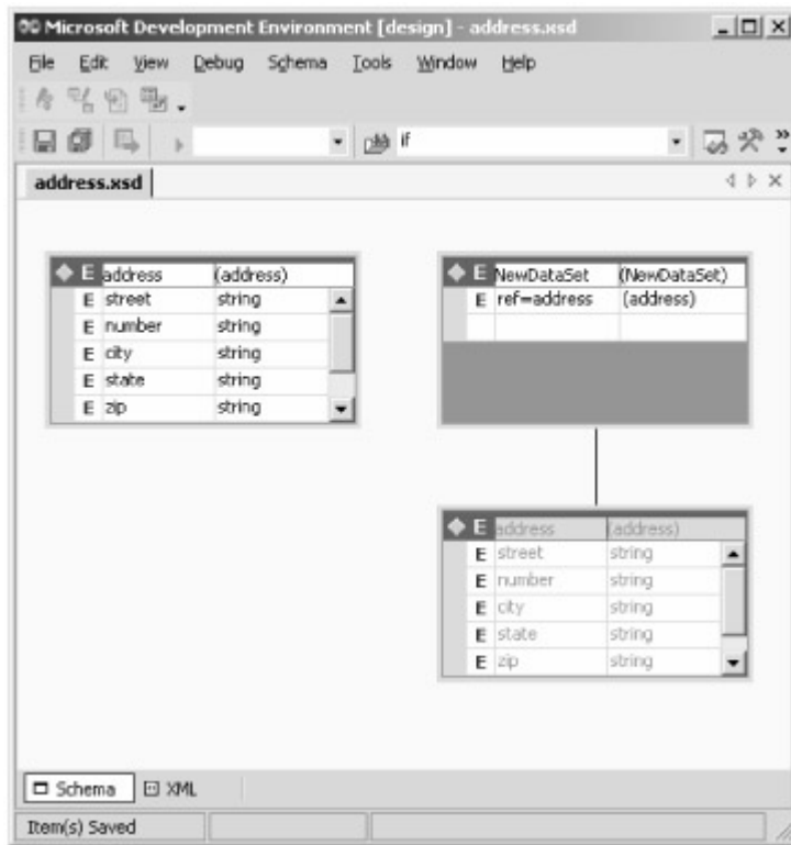
Figure 3-10: The graphical representation of the schema that Visual Studio inferred from the sample document.
