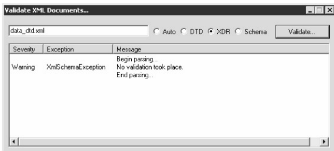
Figure 3-5: The parser has attempted to use XDR validation on a DTD-driven XML document.
