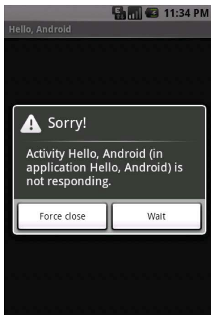
Figure 3–3. The Android “Application Not Responding” dialog
