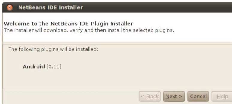
Figure 1–22. Installing the NBAndroid plugin in NetBeans
