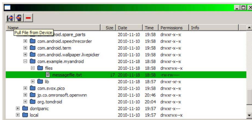
Figure 2-28. The File Explorer window with a view on the file system and the example message file
