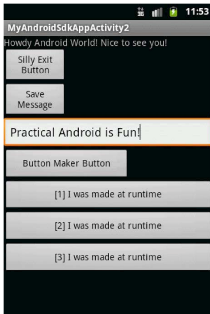
Figure 2–16. The Application with new buttons after pressing the Button Maker Button three times
