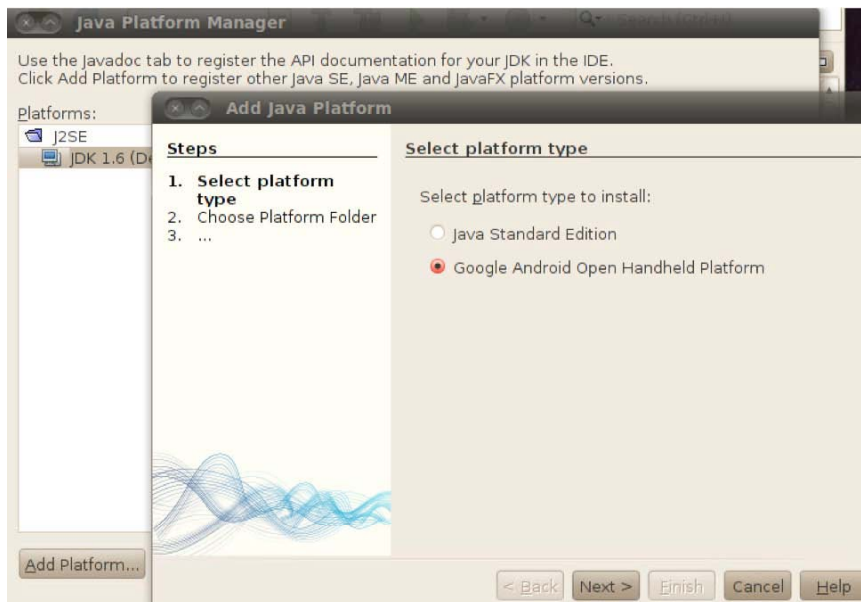
Figure 1–26. Adding the Android Java platform to NetBeans
