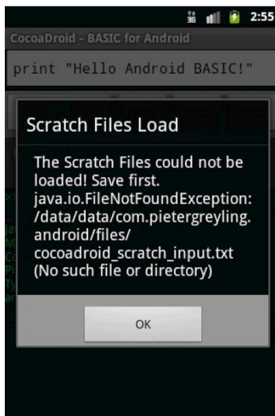
Figure 3–17. Scratch files not found alert
