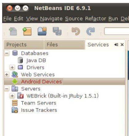
Figure 1-24. The Android Devices node in NetBeans Services
