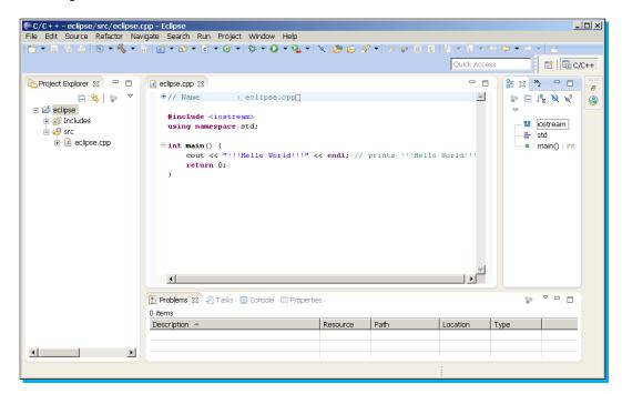
The **Project Explorer** panel is placed at the left-hand side of the window. You can find all the project source files here. The source file editor is placed in the middle part of the window. You can find the messages' output panel at the bottom of the window.
