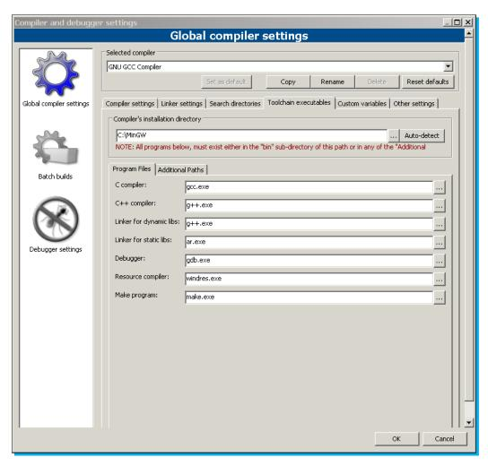
3. Switch to the Toolchain executables tab. Specify the MinGW software installation directory and its utility executables file names.
