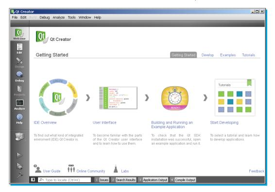
The **Welcome** tab content is placed in the middle of the window. You can see the main system menu at the top of the window. The control panel is placed at the left-hand side of the window. The most commonly used commands are available in this panel. Moreover the icons of different Qt Creator IDE modes (Editor, Designer and so on) are placed here. The messages' output panels are available at the bottom of window.
