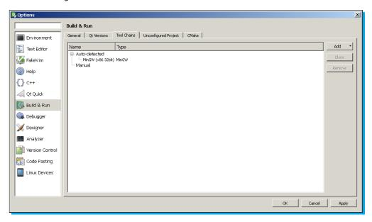
Ot Creator can find already installed MinGW software automatically, but I recommend you manually add it for detailed configuration.
