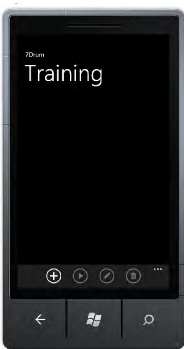
Figure 3-4. The application bar contains four buttons, but only one is enabled.
