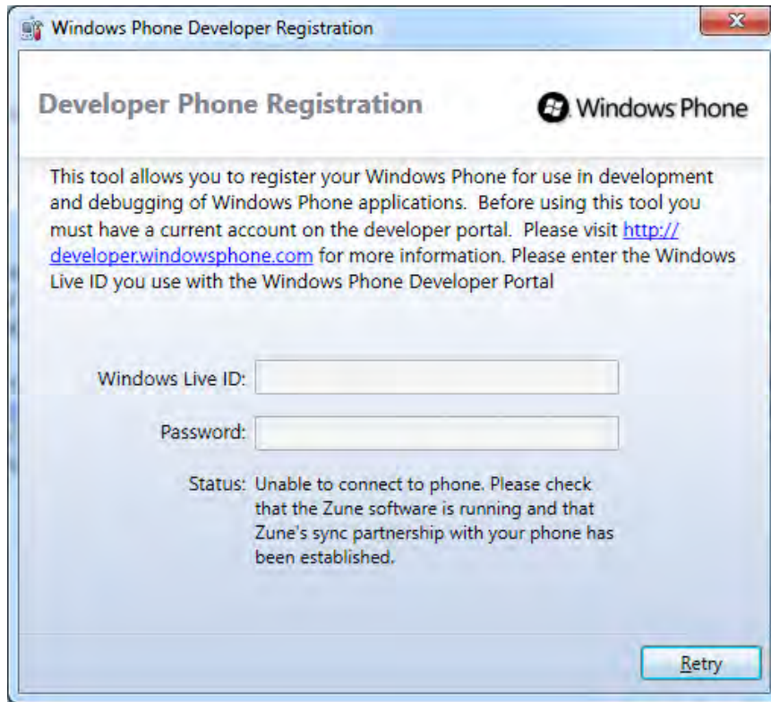
Figure 1-11. The Windows Phone Developer Registration tool used to unlock your phone and deploy applications
