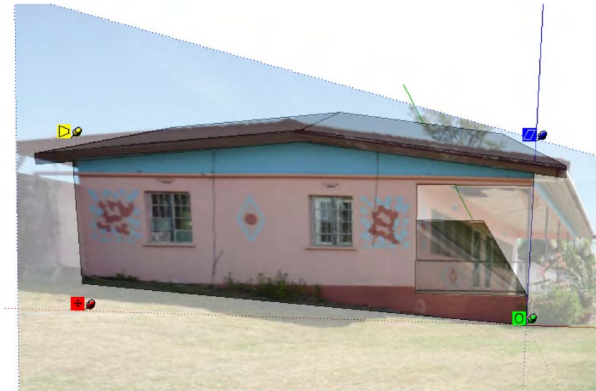
Figure 7–20. In Fixed Pin mode, you can skew, scale, shear, and distort the texture.
