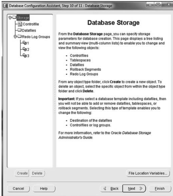
Figure 2.15 Oracle 11g R2: Database Storage (note the redo log groups).
