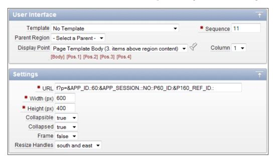
This screenshot shows a typical use of the iFrame panel plug-in with a relative URL referencing another APEX page and containing APEX substitution strings. Notice in the **User Interface** section that the **Template** field has been set to **No Template** because the plug-In will create a panel automatically.
