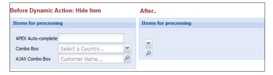
The APEX-generated code for the **Hide Item** dynamic action references the APEX item names, assuming the items are simple DOM elements. For ComboBoxes, this results in the text item component being hidden, leaving the trigger icon visible.
