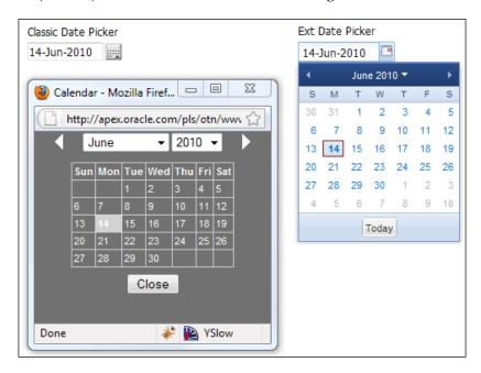
The Ext alternative to this classic date picker is the Ext.DatePicker, a highly configurable component, which dynamically constructs a calendar within the page when the icon is clicked. It also allows you to rapidly scroll through months and years using keyboard shortcuts; it also features auto-complete functionality, allowing you to type partial dates or use alternative date formats, which are automatically converted when you tab out of the field.
