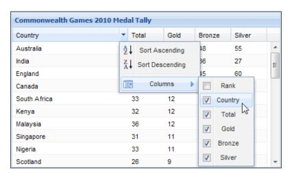
The previous screenshot shows the Total column in its new position, along with a column header menu containing sorting options and a checkbox list of columns to hide or show columns. Notice that the Rank column has been unchecked, and is now hidden.
