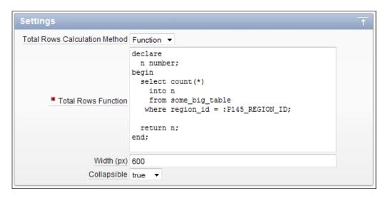
The built-in wwv\_flow\_plugin\_util.get\_plsql\_function\_result function allows developers to use bind variables in exactly the same way as they would for any standard APEX code region.
