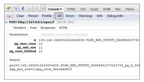
Using this information, we can create an Ext.Ajax.request, passing the same parameters and then capturing the server response.
