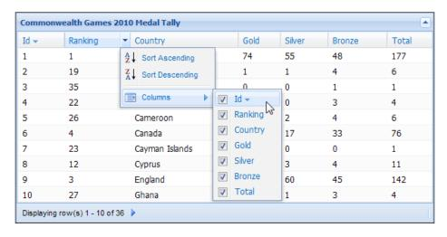
Instead of using the table header to determine the Column model, we can query the APEX metadata for the report for the same information. This is more reliable, and also means we don't need to strip out unwanted elements from the header, just like the sort image and the JavaScript calls to do column sorting.
