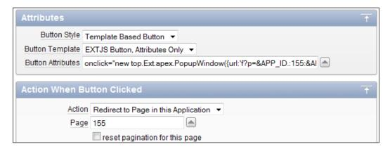
It is also necessary to create a custom button template ExtJS Button, Attributes Only by copying the ExtJS Button template and removing the onclick="#LINK#" reference:
