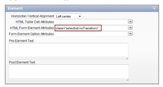
Finally, a check is added to the code to skip select lists with the noTransform class:
