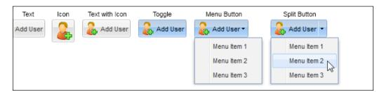
To convert our buttons to Ext buttons, we first need to override the **Ext.Button** object to modify its functionality, in order to allow the button object to be applied to our markup.
