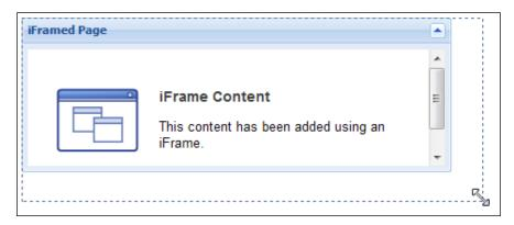
The Ext.Resizable class uses a dashed DIV element as a proxy when sizing using a click-and-drag motion. Once the user releases the mouse click, the iFrame is resized to the new dimensions. Resizing iFrames multiple times as the user moves the mouse is a much more expensive on memory resources than a simple DIV element, so using a proxy element is a sensible solution.
