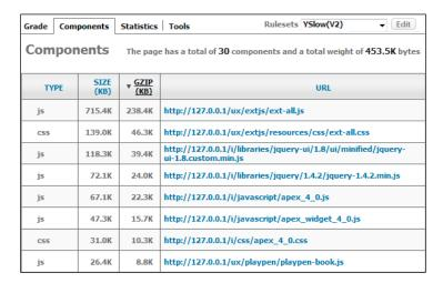
The Firebug YSlow add-on by Yahoo shows the reduced size of page components when gzip compression is enabled. You can see the Ext library **ext-all.js** has a gzipped size of **238.4K** compared with **715.4K**, or roughly a 70% reduction in size.
