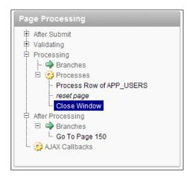
The Close Window process completes before the After Processing section where page branching occurs. It does this by rendering a very small HTML page and then terminating any further processing by the APEX engine.
