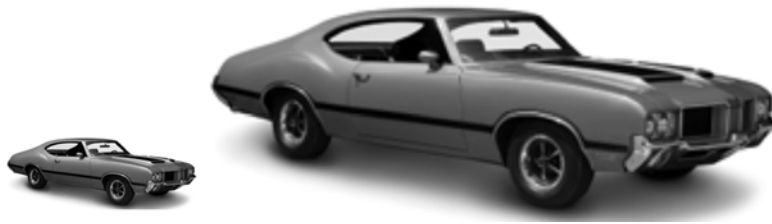
Figure 6.7 Image enlargement using bilinear interpolation
