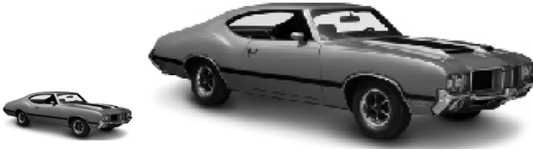
Figure 6.4 Image enlargement using nearest-neighbor interpolation
