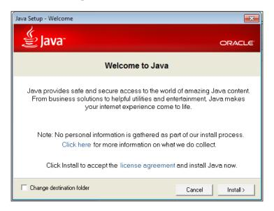
We can suppress this by passing the appropriate flags to the executable via the InstallCommand attribute. In this case, for a silent install, we would pass the /s flag, as shown in the following snippet:
