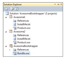
When you build the solution, the bootstrapper project will compress the two MSIs into its output executable, as shown in the following screenshot:
