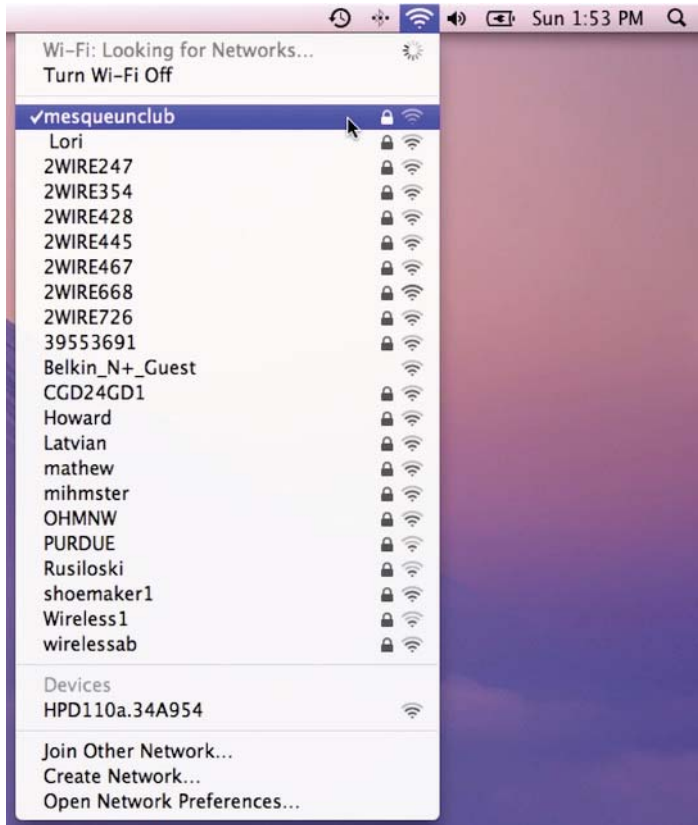
Figure 8–5. The Wi-Fi status menu on the menu bar provides you with the information and tools to connect to a Wi-Fi network without using the System Preferences.
