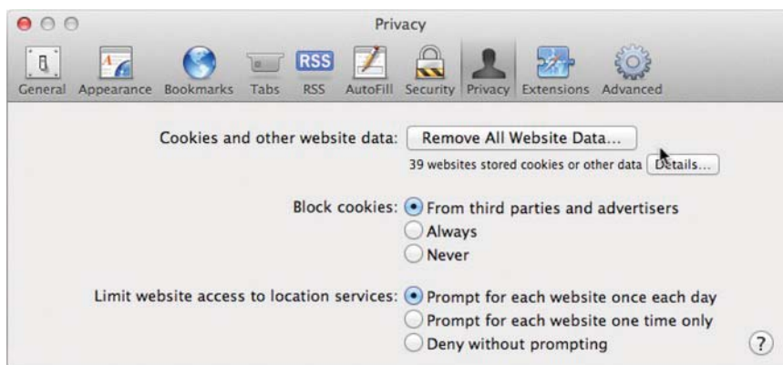
Figure 9–10. The Privacy tab in Safari's preferences allows you to control what sort of data is collected and shared with Safari. The options here allow you to determine what cookies you would like to block and how location data may be used. You can also remove selected or all data Safari has collected from here.
